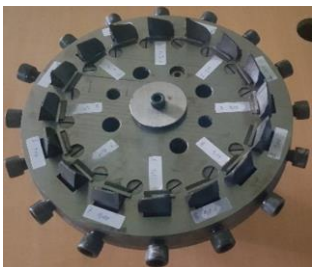
Figure 2. Kyocera end mill of Gleason spiral bevel gear with an alloy
